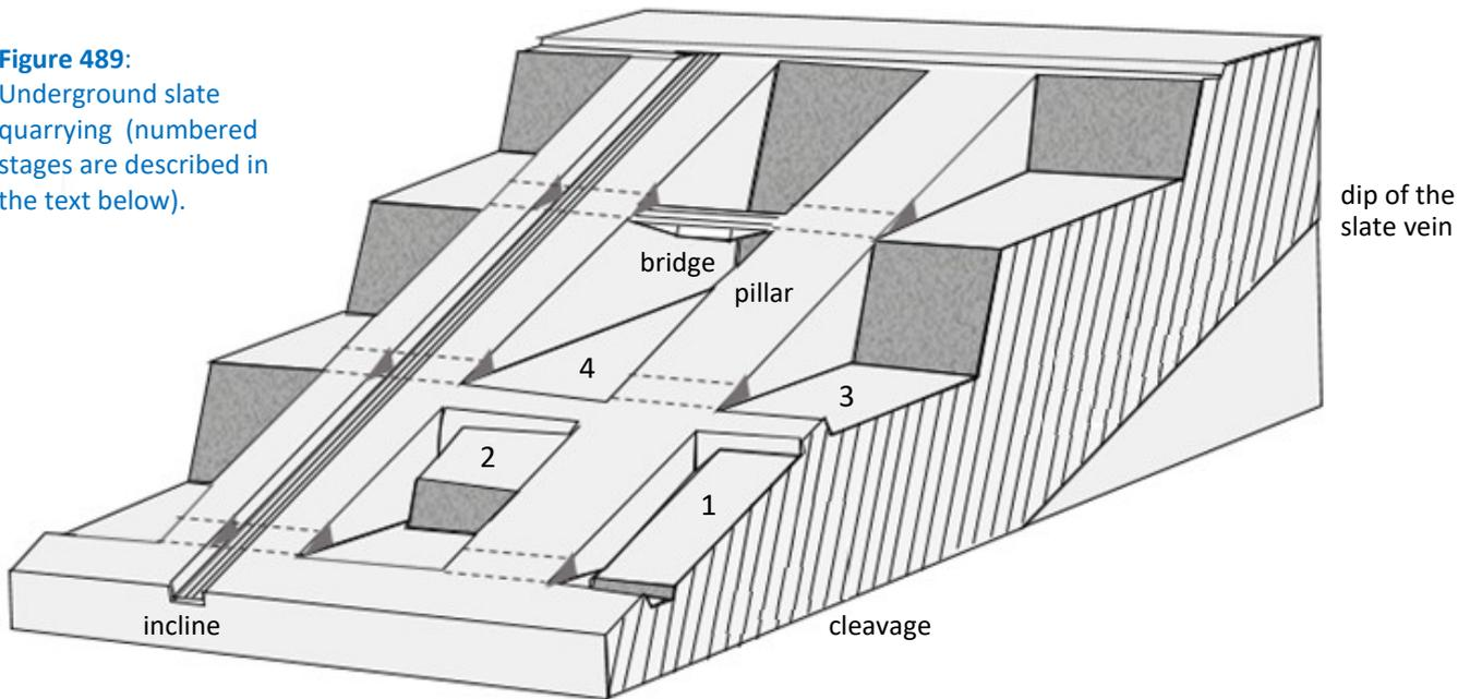
An access tunnel or **adit** was driven from the valley side to reach the slate vein. From this point, an incline could be cut below the roof of the vein to provide a transport route for the removal of slate (fig. 490).
