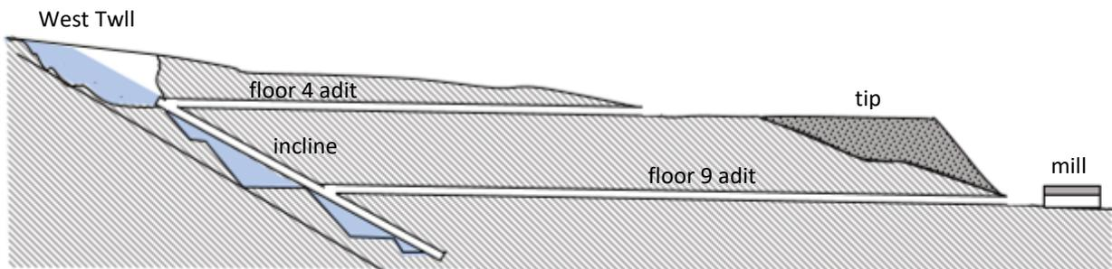
**Figure 491:** Diagrammatic cross section of the Rhosydd quarry workings. The Old Vein is shown in blue.
