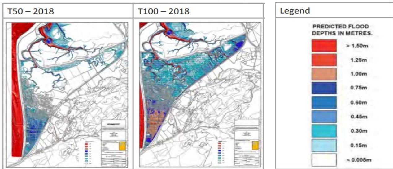
**Figure 38:** Computer models for flooding of Fairbourne in 2018 for storms of 50 year and 100 year frequency.
