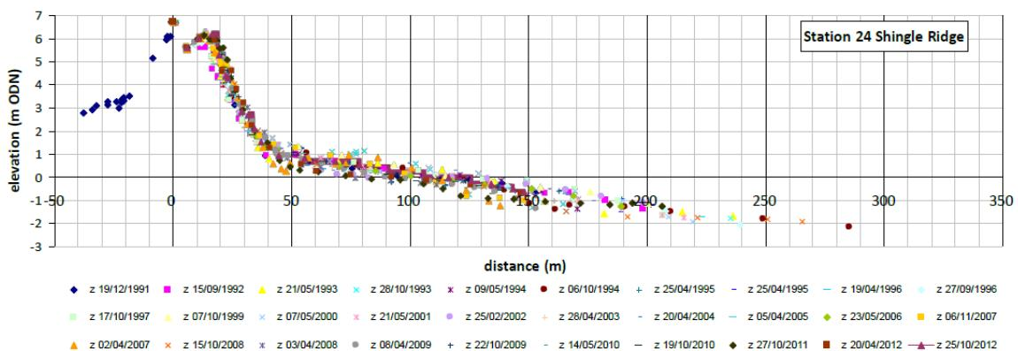
**Figure 17:** Monitoring of the storm beach profile in front of Fairbourne village over the period 1991 – 2012 (Phillips et al., 2017).
