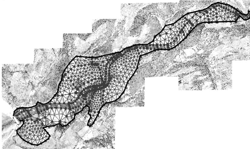
**Fig. 14.** Finite volume discretisation for the Mawddach estuary, based on a bathymetric survey (Olding Smee Oberman Associates, 1985) and natural vegetation zones delineated from air photography.
