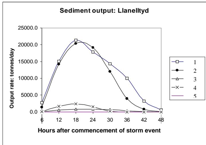
**Fig. 11** (left). Area of gravel deposition at the head of the estuary. (right) Modelled output of sediment from the River Mawddach into the tidal estuary during the 3 July 2001 flood event. Legend numbers refer to sediment classes: 1, silt-coarse sand; 2, very coarse sand-fine gravel; 3, medium-coarse gravel; 4, very coarse gravel-cobbles; 5, boulders.
