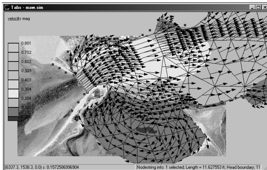
**Fig. 12.** RMA2 simulation of a flood tide entering the Mawddach estuary.
