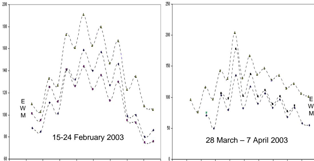
**Fig. 10.** Correlation of tidal maximum heights at the estuary mouth (E) and at the river tidal limits of the Mawddach (M) and Wnion (W).
