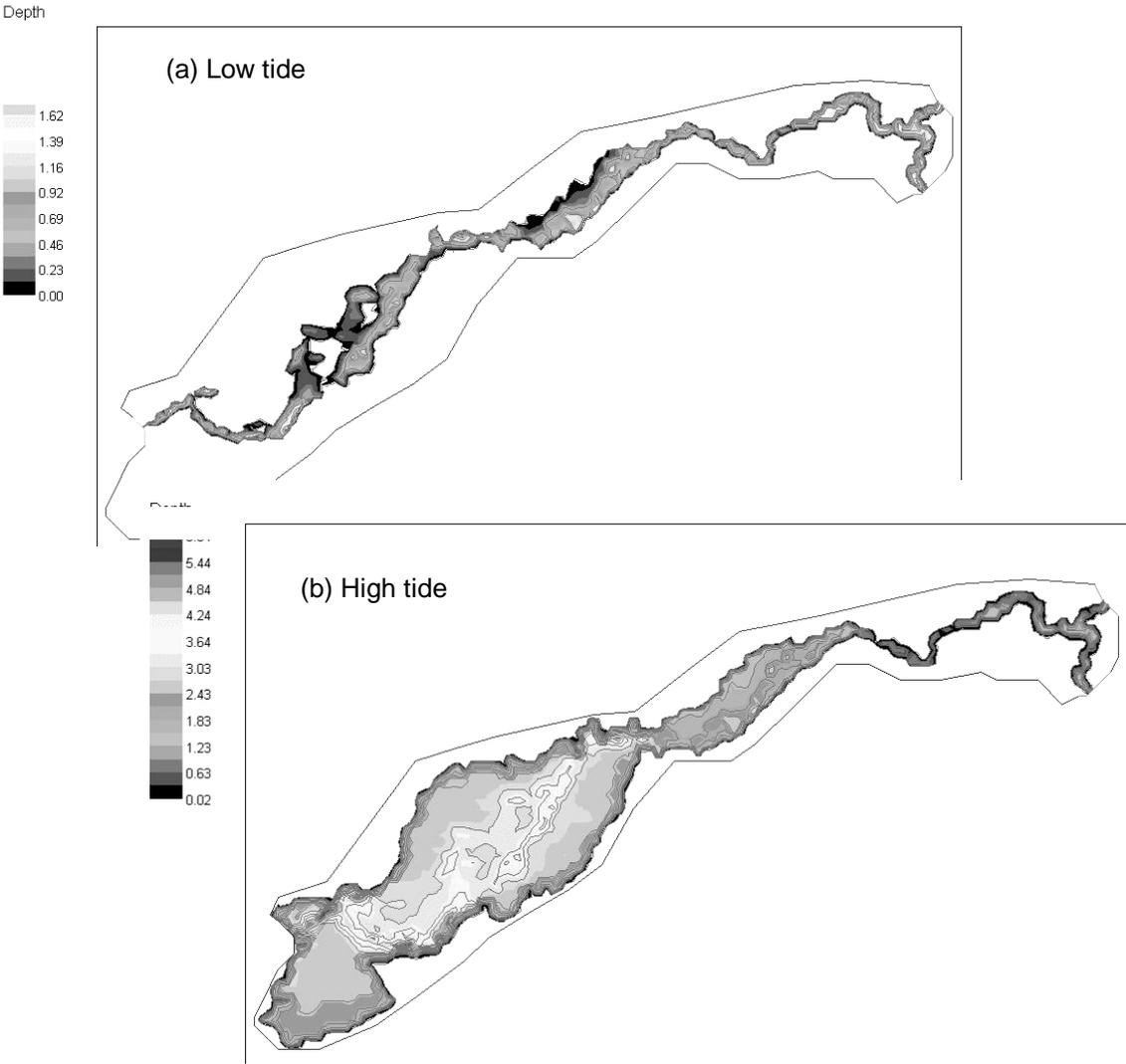
**Fig. 13.** Simulation of a 4m tide for the Mawddach estuary. Extent of the computation domain is outlined.
