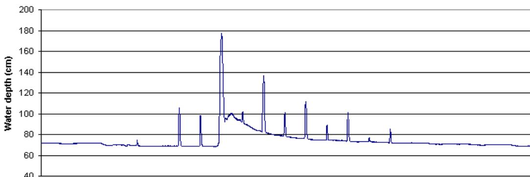
**Fig. 8.** River Wnion: hydrograph near the tidal limit for the period 28 March – 8 April 2003
