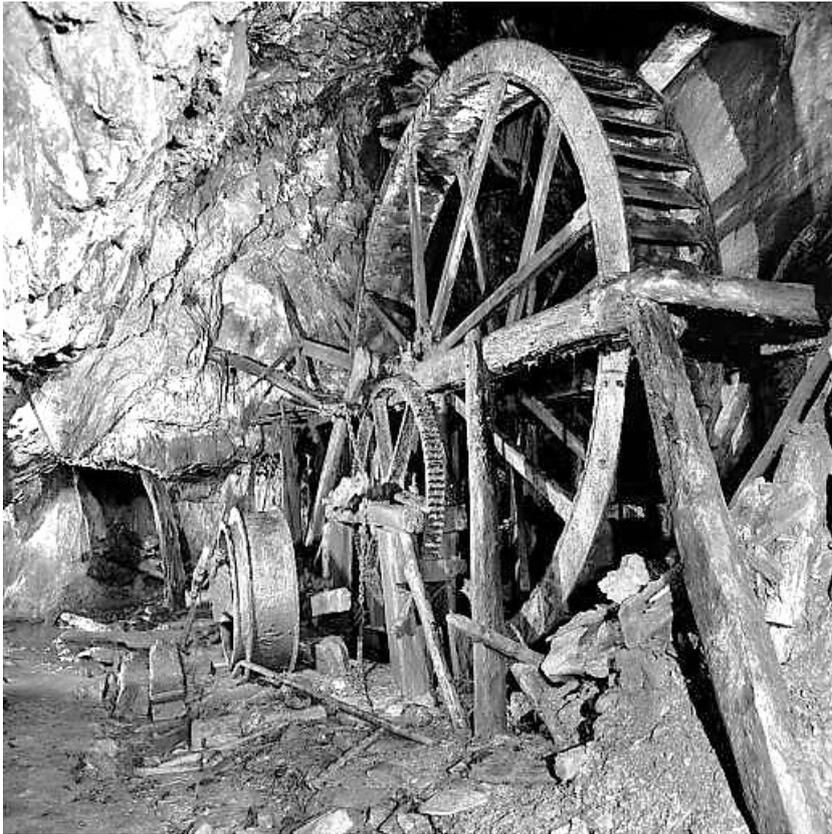
**Figure 154:** Underground water wheel, Ystrad Einion mine.
